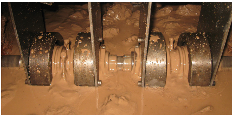
Mudslurry test rig
